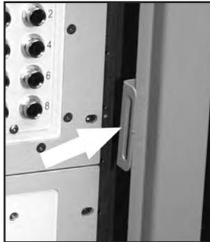
Figure 4. Cabinet door latch plate.
