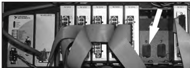
Figure 7. NI chassis next available slot, frequency module always to the Right.
