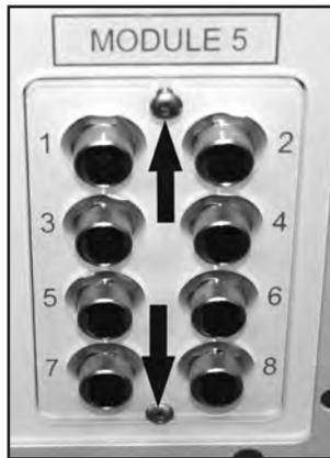
Figure 8. Module fixing screws.
