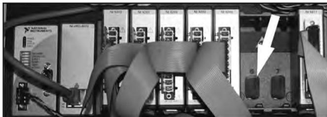
Figure 7. NI chassis next available slot, frequency module always to the Right.
