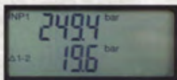
Pressure 1 Differential pressure
