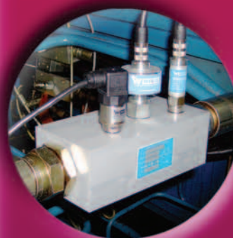
CT Turbine flow meter
