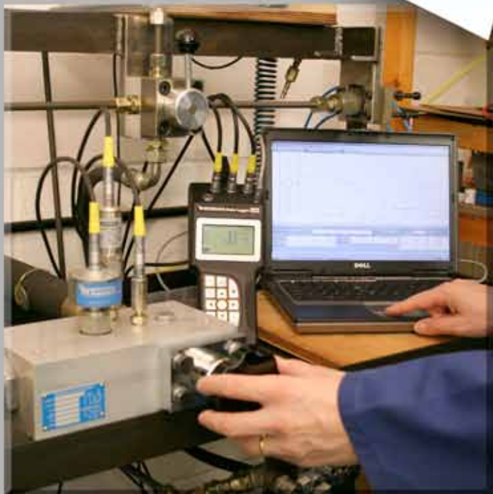
Faultfinding on a hydraulic test bench with the HPM540 connected to a PC via USB
