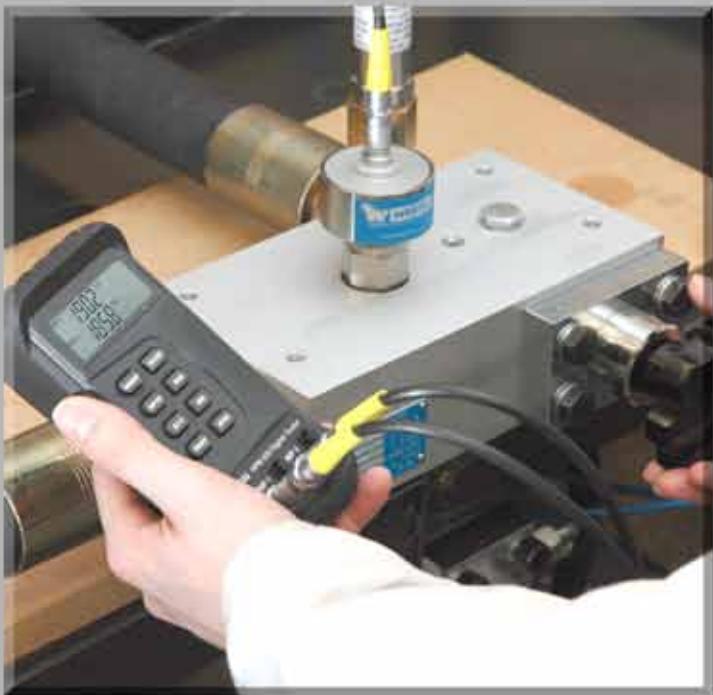
Testing pump flow and pressure with the HPM420
