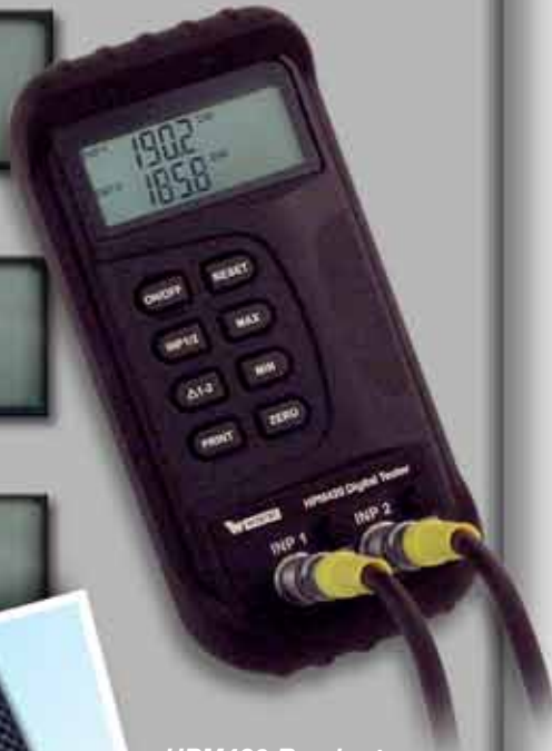
HPM420 Readout, 2 inputs
