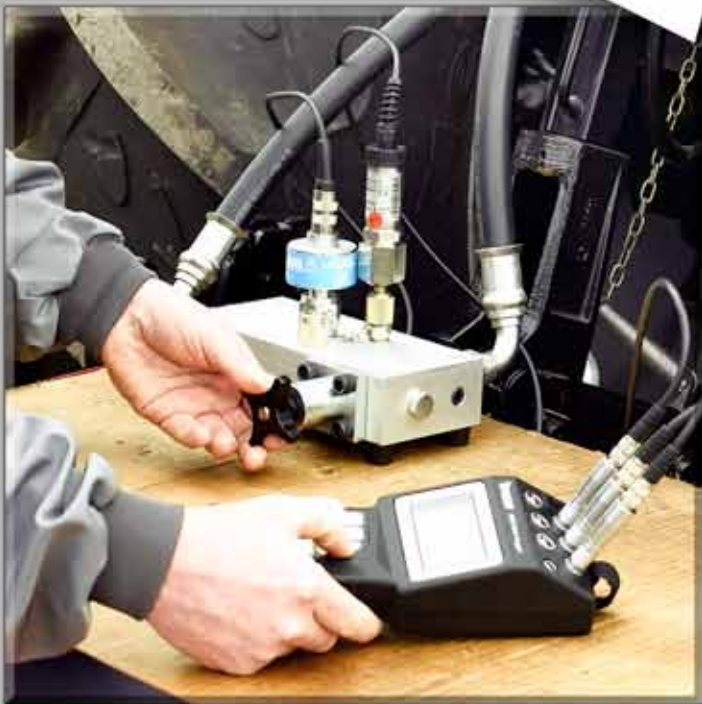
Faultfinding on a tractor with the HPM460
