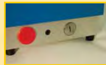
Integral safety burst disc holder is shown on the right of the above picture.
